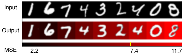
Figure 1: Limitation of novelty detection using image reconstruction error. Top: Input images. Middle: Output images of adversarial autoencoder (AAE). Bottom: mean squared error (MSE) of all images. We set the images of digits of 0-8 and 9 as normal and novelty, respectively. Since mean of novelty scores among the image of digit 9 (novelty class) is 7.4, MSE values of normal image bigger than 7.4 lead to wrong novelty detection.
